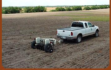
Electrical conductivity soil sensor. (Photo courtesy of Veris Technologies)
