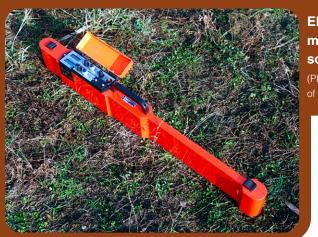
Electromagnetic soil sensor. (Photo courtesy of Geonics Inc.)
