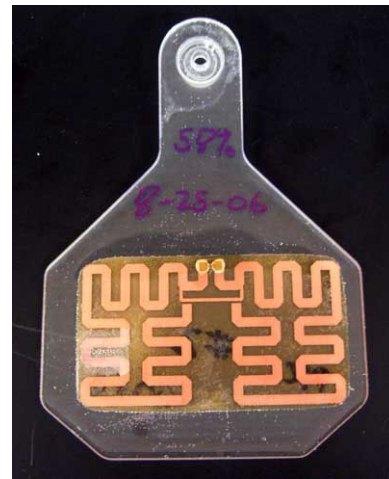
Fig. 1. Cattle tag with embedded passive RFID tag.
