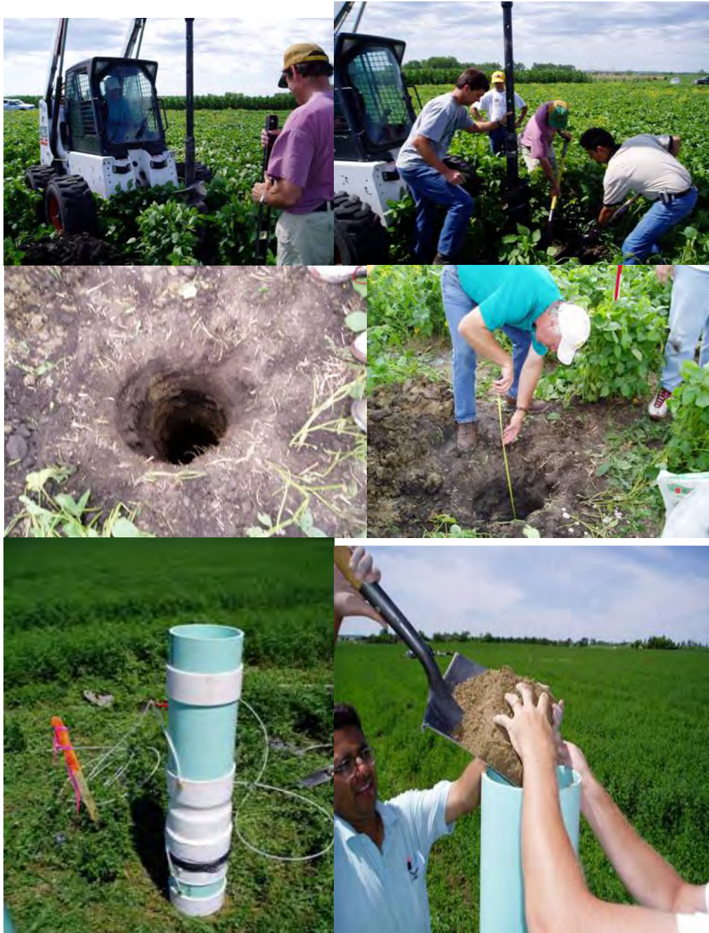
Figure 6a Sequential steps of flux meter installation in the field
