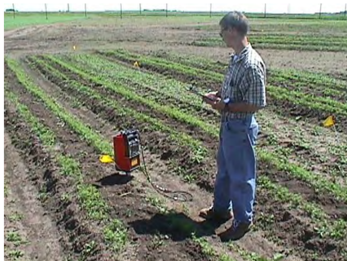
Figure 8 Neutron probe readings for soil moisture monitoring
