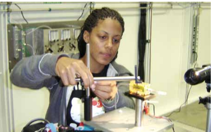
Haleigh Eubanks prepares a caterpillar for X-ray imaging at the Advanced Photon Source at Argonne National Laboratory. The caterpillar is in a respirometry chamber so they can measure expired carbon dioxide and synchronize that to X-ray videos.
