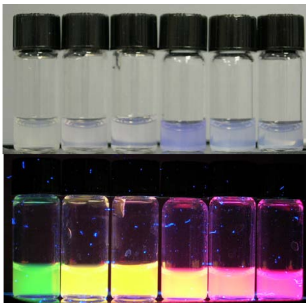
Figure 6. Fluorophore-conjugate doped nanoparticles illuminated under 365 nm UV light (From left to right are nanoparticles doped with conjugates from 1 to 6 listed in Table 1).
