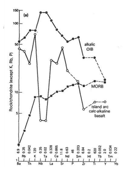
Typical spiderdiagram pattern for mid-ocean ridge (MORB), oceanic-island (OIB) and island-arc basalts normalized according to Thompson et al. (1984). Values of the normalization constants used are given as ppm at the foot of the diagram.
