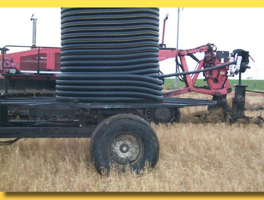
Figure 3. Installation of tile drainage in progress in Ramsey County along state Highway 17 near Edmore, N.D.
