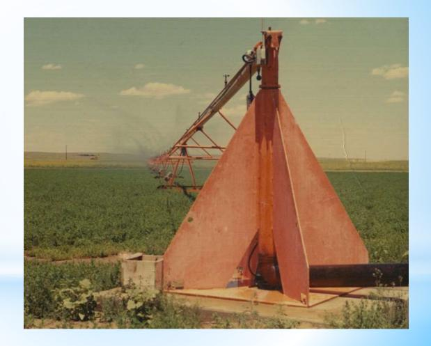
During the 1960's many experimental versions of the center pivot were developed. Most were powered by the water pressure in the delivery pipe.
