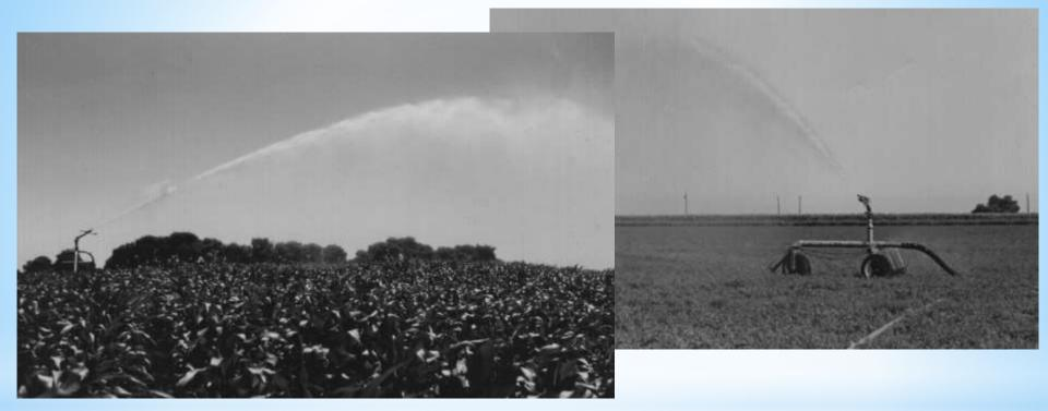
Volume sprinklers (commonly called "Big Guns") have been used from the 1950's up to the present day. They can throw water from 150 to 300 feet depending on nozzle size, pressure at the sprinkler head and angle of throw.
