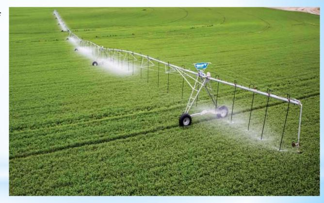
Currently, center pivots are used on almost all the sprinkler irrigated land in ND. Surface irrigation is still used in the areas developed during the 1940 - 1950's.
