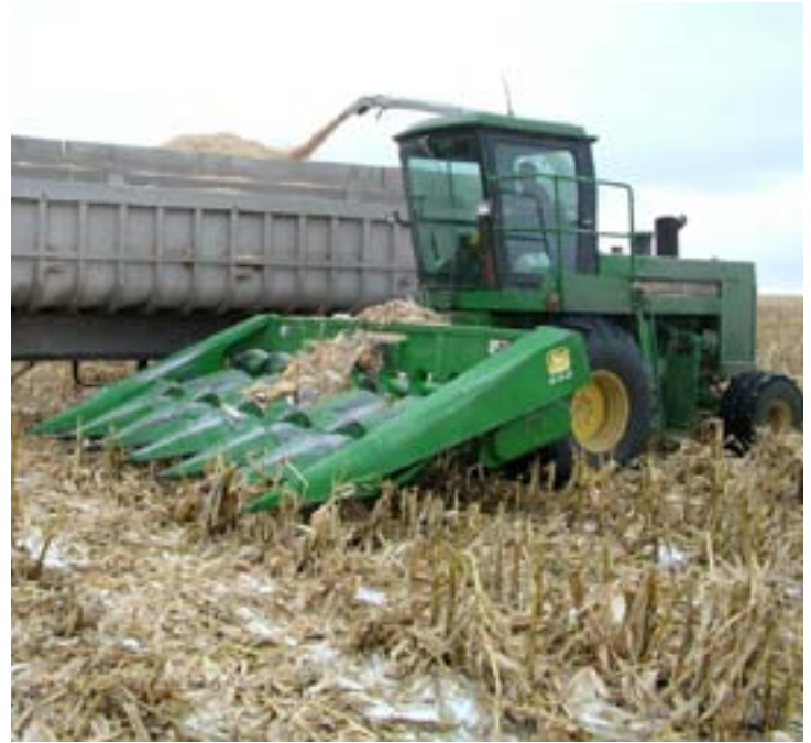
Figure 2. Harvesting snaplage in northeastern North Dakota using a self-propelled forage harvester and a snapper head.
