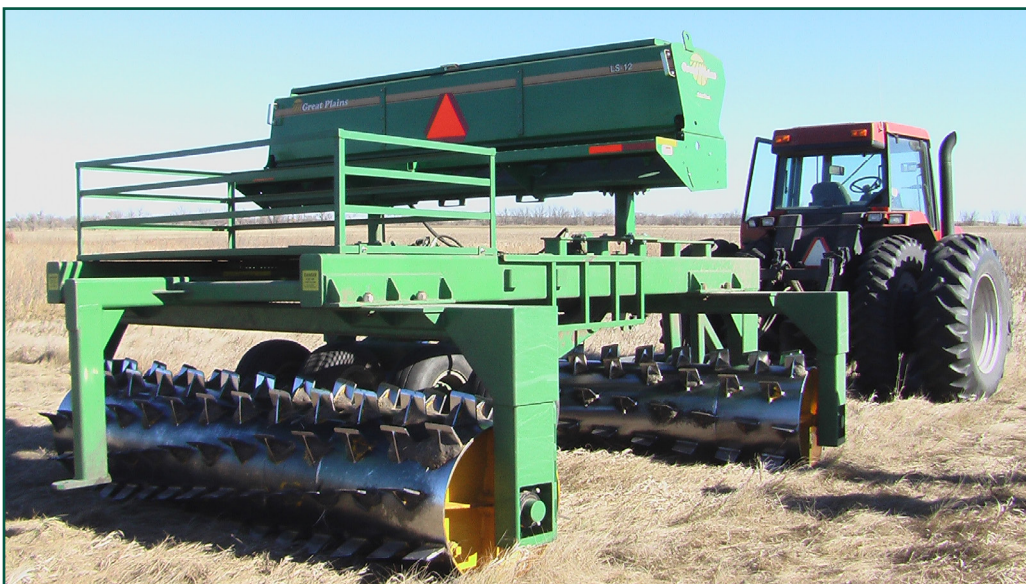
Aerator rollers can be used to cut residues into manageable lengths and flatten animal mounds prior to no-till planting.
