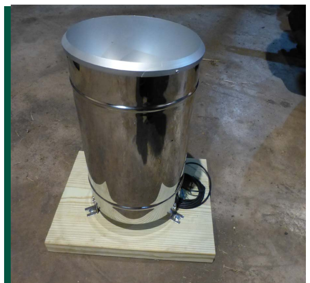
Figure 4. Rain gauge sensor. (John Nowatzki, NDSU)
