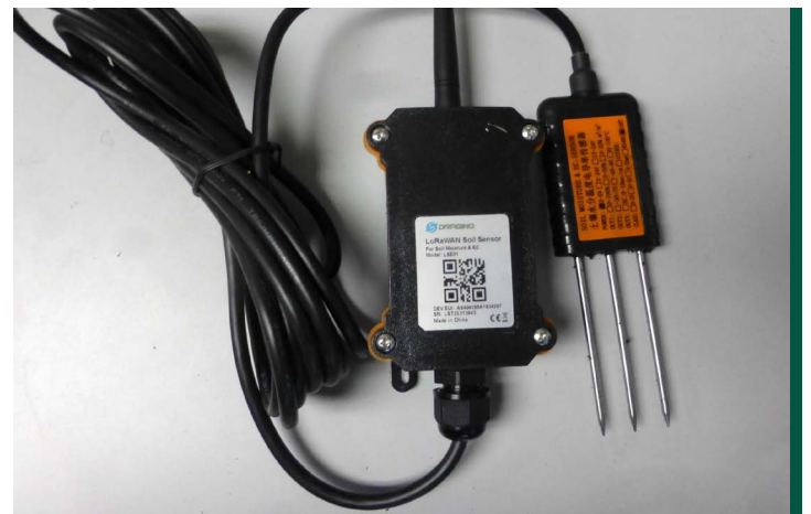
Figure 1. Soil moisture sensor. (John Nowatzki, NDSU)
