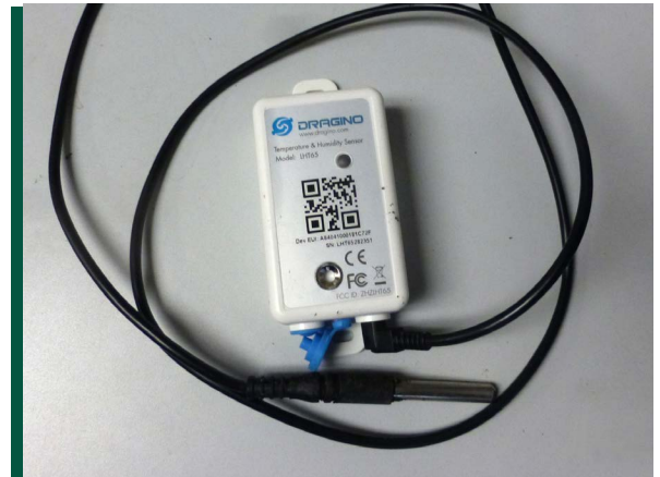
Figure 2. Temperature sensor. (John Nowatzki, NDSU)
