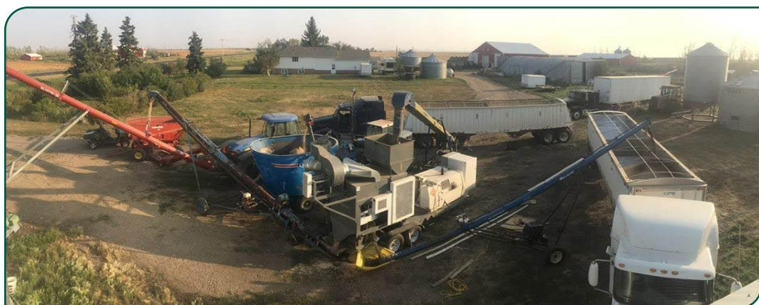
Figure 3. Separating and cleaning pea-canola intercrop using a portable seed cleaning unit. Mixed grain enters the cleaner via the auger in the middle, clean canola exits via the blue auger on the right, clean pea exits via the brown auger on the left, and screenings are collected in the round blue tub behind the cleaning unit. [M. Jacobs]
