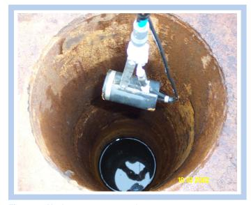
Figure 4. Underwater camera about to be lowered into a well to look for problems in the casing and screen.
