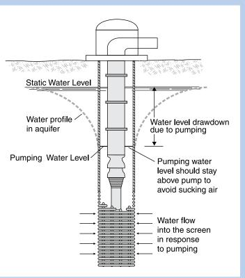
Figure 2. Side view of pumping irrigation well.
