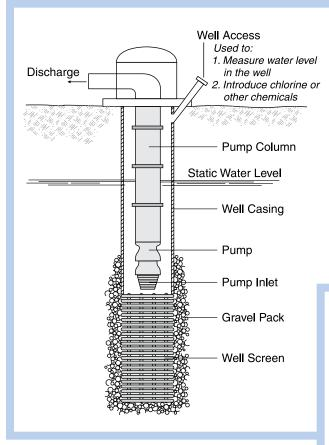
Figure 1. Typical irrigation well and pump.
