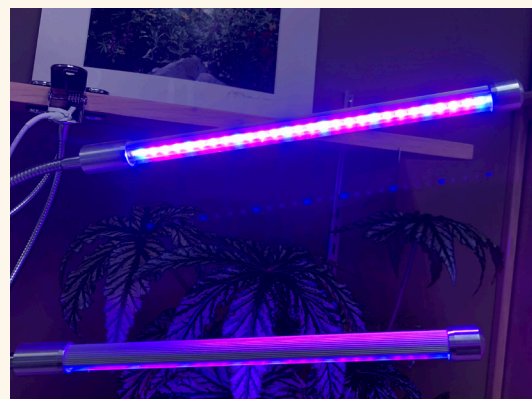
Fig. 2. Photo of a red and blue LED grow light that is being used for supplemental lighting in an office.
