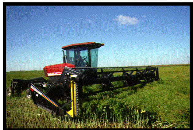
Figure 8. Swather equipped with vertical cutter bar.
