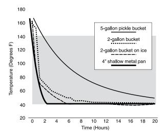
Acceptable cooling occurred when chili (at a depth of 2 inches) was placed in a shallow metal pan in a 40 F cooler. Chili (at a depth of 10 inches) in a twogallon plastic bucket cooled within acceptable limits only when an ice bath was used and the mixture was stirred periodically.
