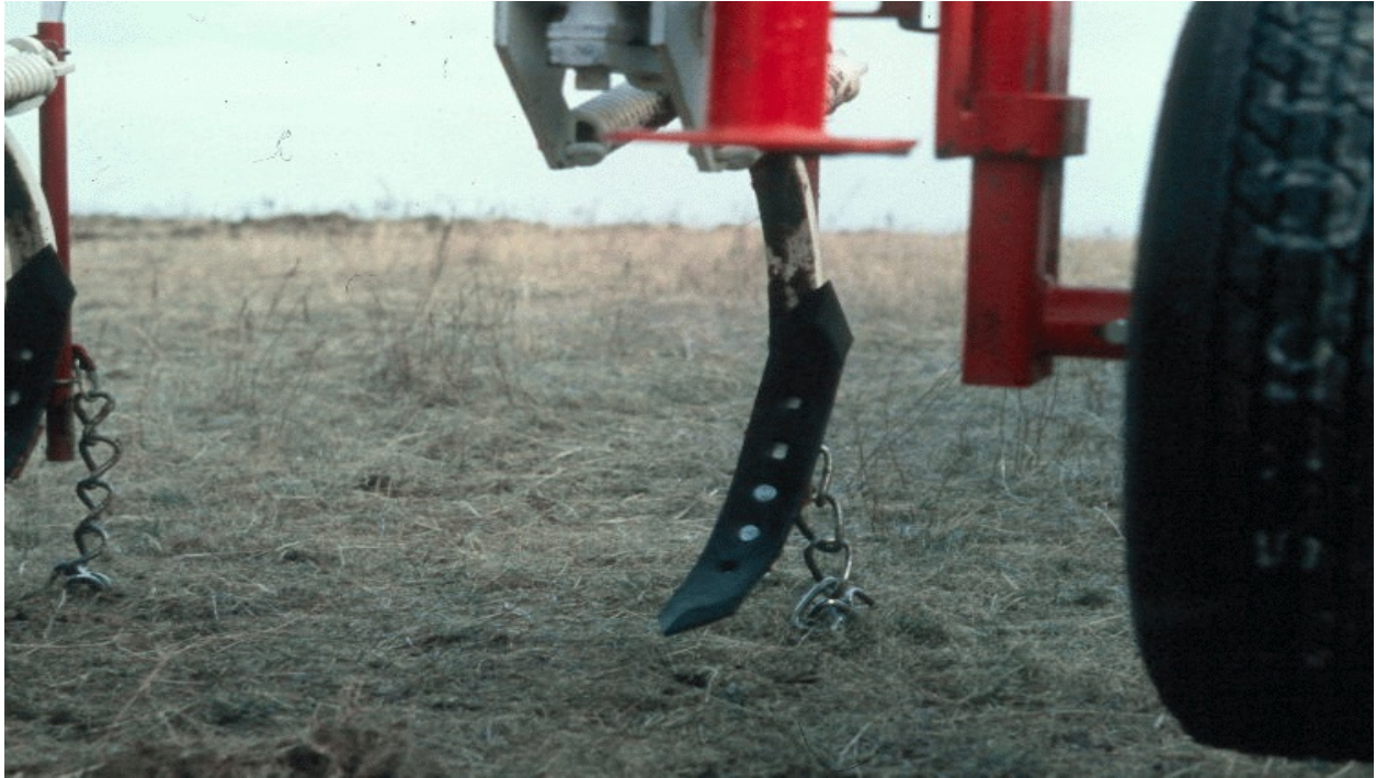
Fig. 3. Three-inch twisted chisel plow shovel.
