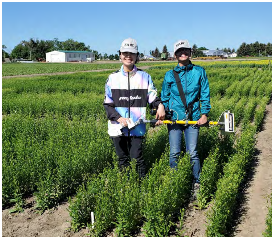
Yi and Shreya performing remote sensing for the measurement of camelina canopy NDVI.
