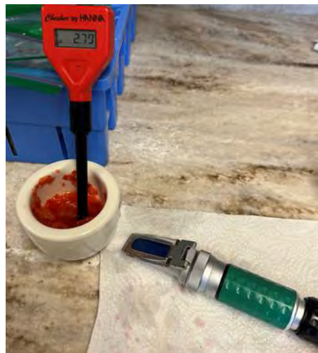
Brix and pH value recorded using Veegee refractometer and Checker portable pH. Photo by Rojee.
