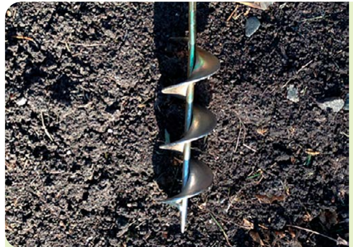
Figure 3. A 3-inch bulb auger attaches to an electric drill and can be used to drill vertical pockets in the soil.
