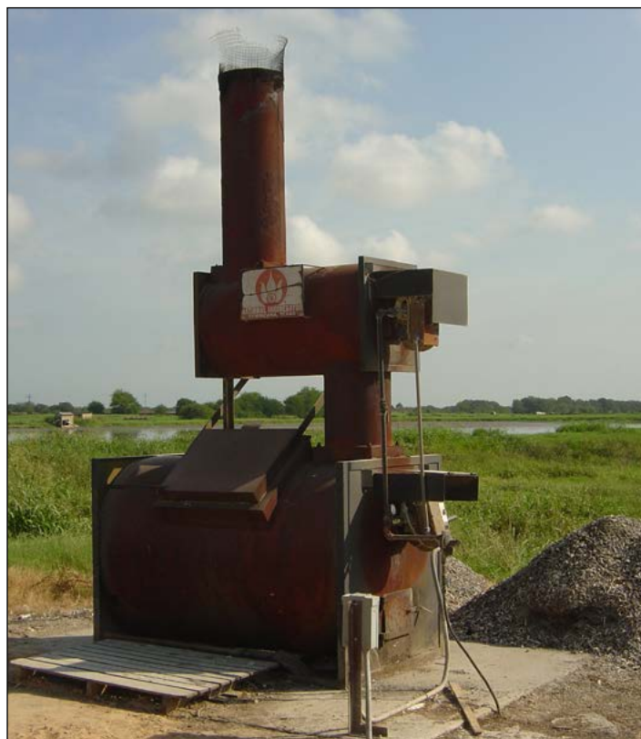
Figure 1. Incinerator for managing poultry carcasses. (NDSU photo)
