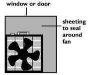
Place fan facing out in a window or door and seal the rest of the opening.
