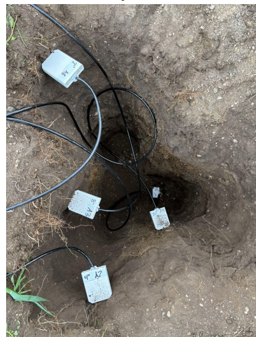
Image 3: A soil pit with the five soil moisture & temperature sensors
