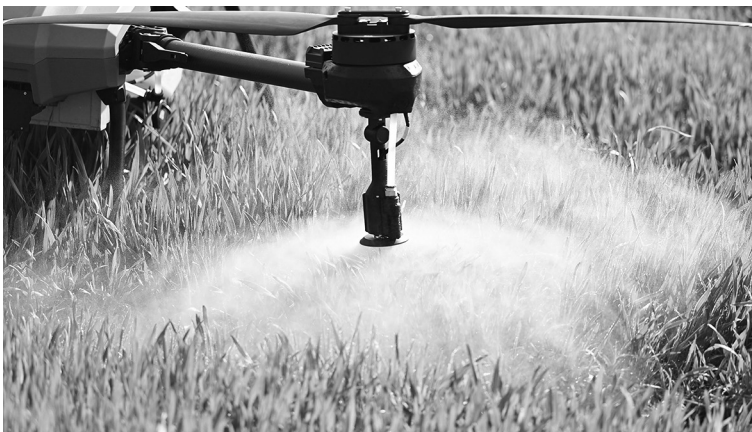
Figure 30. Closeup of a spray drone that features a rotary atomizer for droplet generation. Photo by DRONE EFT on Unsplash.
