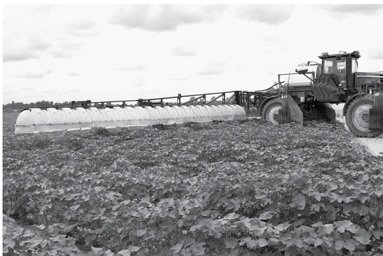
Figure 27. Hooded spray boom. Photo courtesy of Willmar Fabrication, LLC.
