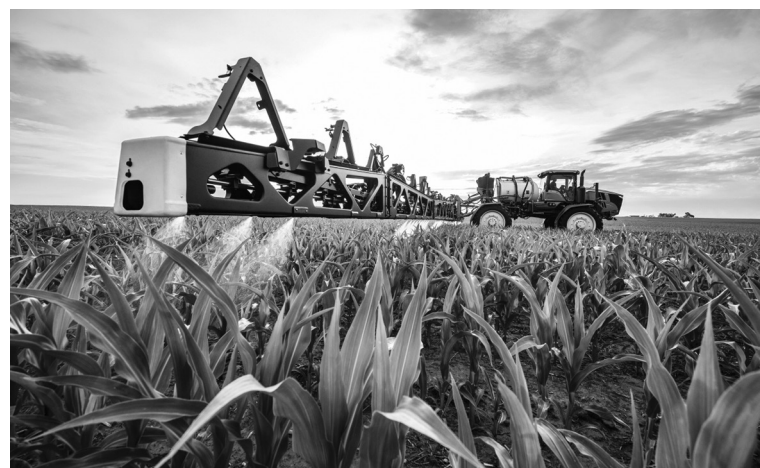
Figure 29. A sense-and-act sprayer. Photo courtesy of John Deere.
