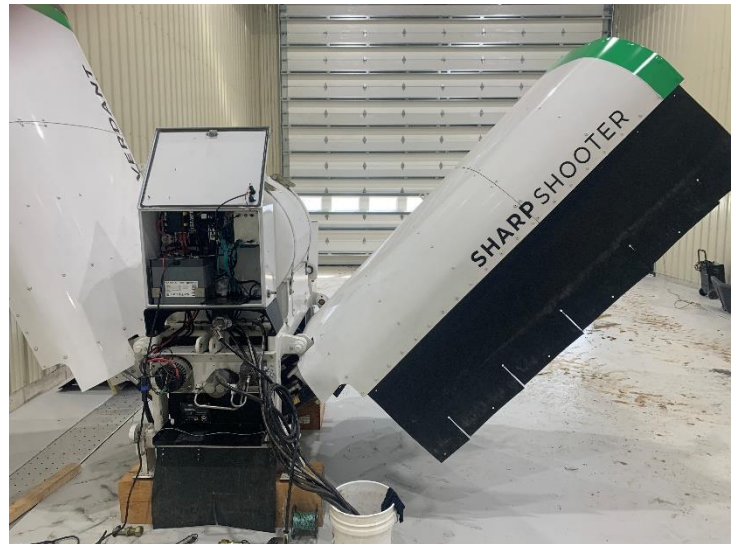
The Verdant Robotics Sharp Shooter uses AI technology to differentiate between crop and weeds, aiming a dose of herbicide at target weeds.
