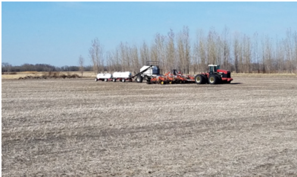
Figure 10.16. Seeder configured for one-pass seeding with anhydrous ammonia application, near Minot, ND. (NDSU photo)
