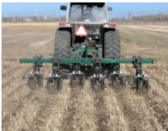
Figure 10.13. Maverick™ shank strip-till unit operating at Carrington REC. (NDSU photo)
