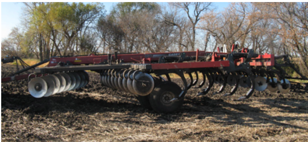
Figure 10.3. A disk ripper with residue cutting disks out front, deep depth shanks behind, then smaller disks to smooth soil behind. (DeJong-Hughes & Daigh, 2021)
