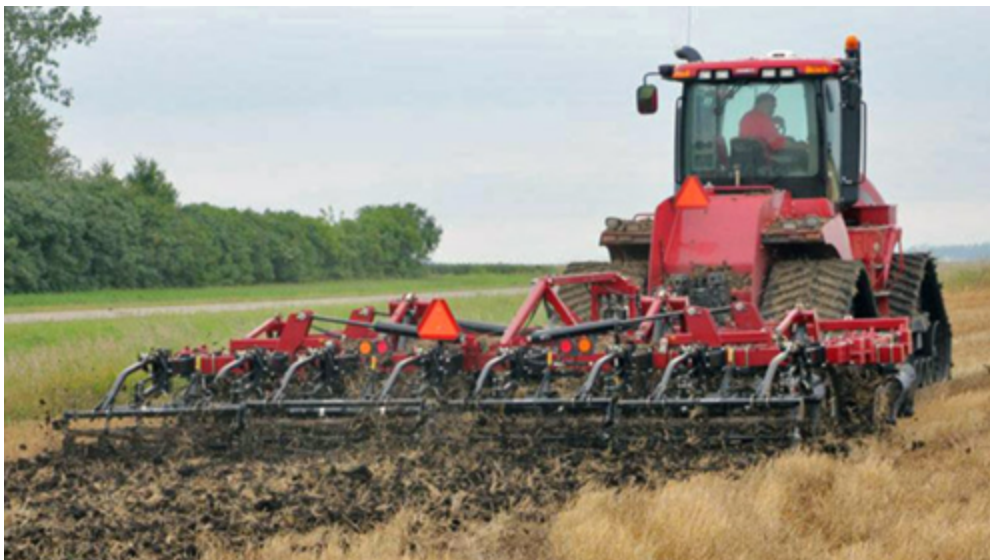
Figure 10.5. Chisel plow in small grain residue. The back gang consists of rolling baskets that tend to crush clods brought to the surface by the chisel plow, enabling easier seedbed preparation the following spring. (DeJong-Hughes & Daigh, 2021)
