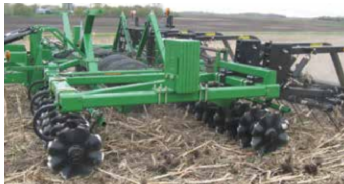
Figure 10.10. Vertical tillage unit showing nearly vertical wavy coulters accompanied by a tine harrow. (DeJong-Hughes & Daigh, 2021)
