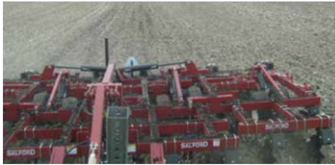
Figure 10.11. Vertical tillage implement being used in the field. Residue remains at or near the surface but at less coverage than untouched residue to the left. (DeJong-Hughes & Daigh, 2021)
