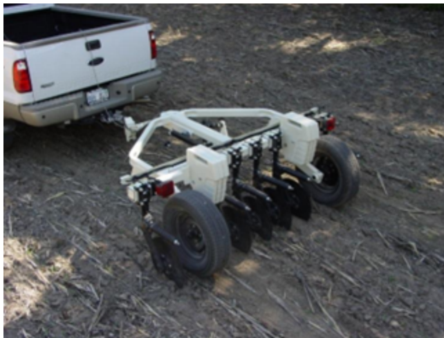
Figure 12.10 Veris™ electrical conductivity sensor, courtesy of Veris Technologies, Salina, KS.
