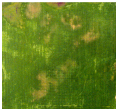
Figure 12.8 Valley City 40-acre field aerial image taken from an airplane flying at 5,000 feet above the soil surface using color Ektachrome film.
