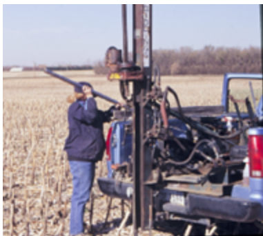
Figure 12.5 Use of a pickup bed hydraulic system in the field to sample deep depths.
