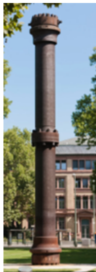
Figure 15.6 Original Haber-Bosch ammonia reactor, BASF complex, Ludwigshafen, Germany (NDSU image)
