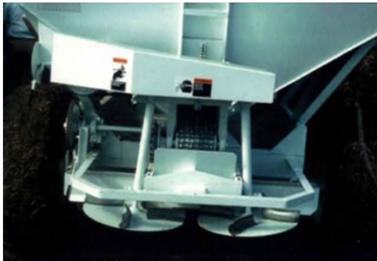
Figure 28.11 A Spinner-type dry fertilizer spreader. This method of application is still commonly used by farmers. Care should be taken when applying, considering that urea does not throw as far as MAP or potash due to its low relative density. If using a blended product of urea with something else, ‘splitting the middles’ would be wise to avoid both over application and under application strips. This means if the width of the throw is 50 feet, the driver should set the spreader to half rate, and drive 25 feet between passes. NDSU image
