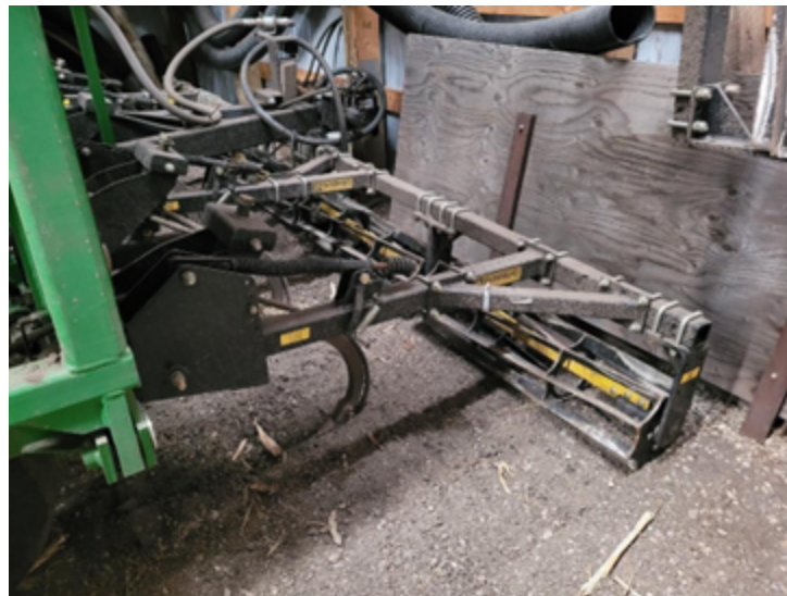
Figure 28.8 Anhydrous ammonia applicator using spike shanks and a rolling basket to cover the application trench. NDSU image
