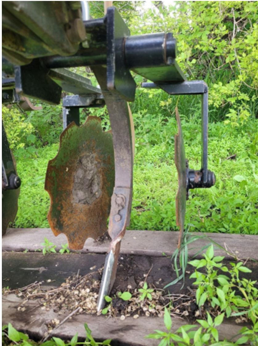
Figure 28.9 Ammonia applicator using adapted ammonia knives on chisel plow shanks, with rolling discs behind to cover the trench. NDSU image
