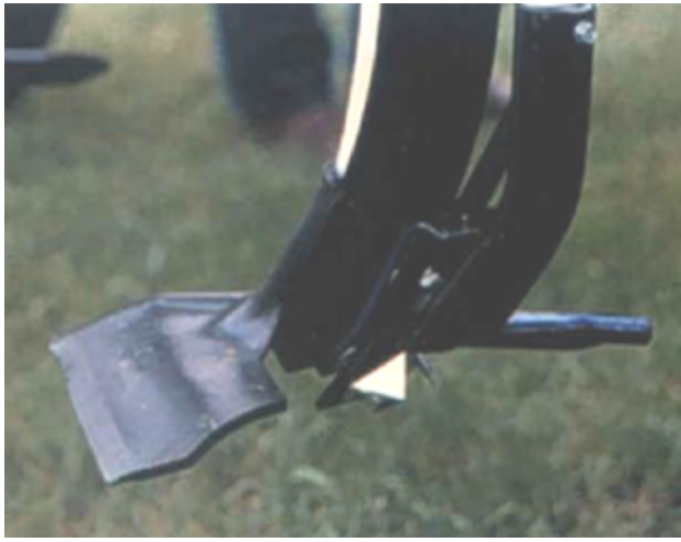
Figure 28.6 and Figure 28.7 Two common methods for introducing anhydrous ammonia into the soil to a depth of at least 3 inches.
