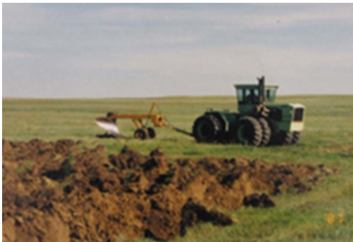
Figure 8.12. A 4-foot plow utilized to incorporate deep native gypsum into surface sodic soils. (NDSU photo)
