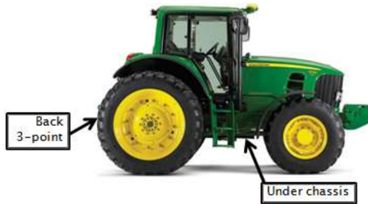
Figure 4.3 - Displays other possible locations for the ballast to be placed.
