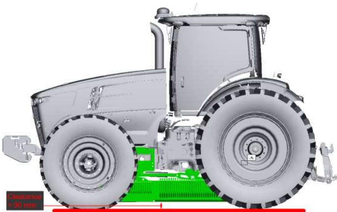
Figure 8.4 - Under-Belly design using modified suitcase weights.
