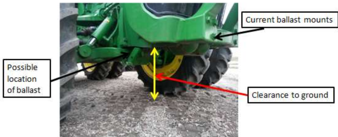
Figure 4.1 - Shows clearance for front end of tractor and underside
