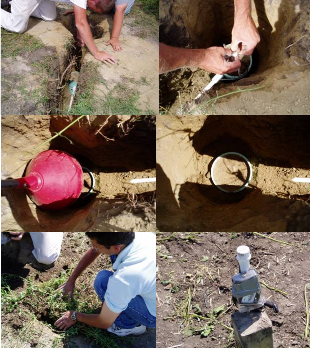
Figure 6b Sequential steps of flux meter installation in the field
