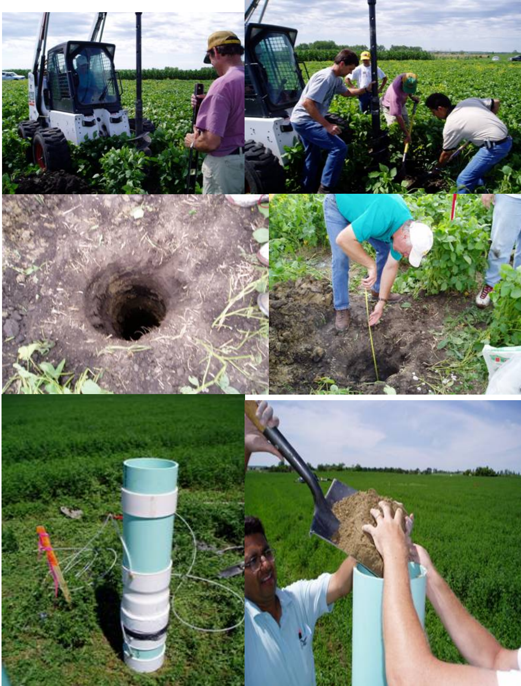
Figure 6a Sequential steps of flux meter installation in the field
