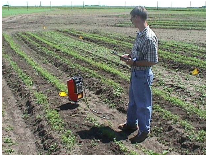
Figure 8 Neutron probe readings for soil moisture monitoring
