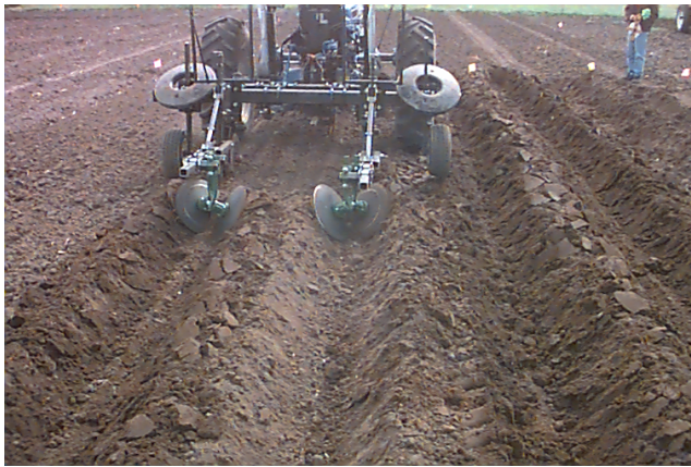
Figure 2. Furrow formation in progress with the modified subsurface drip irrigation plow in 2000.
