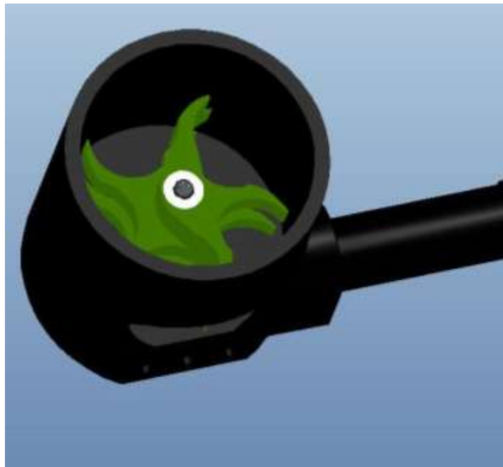
FIGURE 9 - ROTATING SEPARATOR OF A PAINTBALL GUN.
