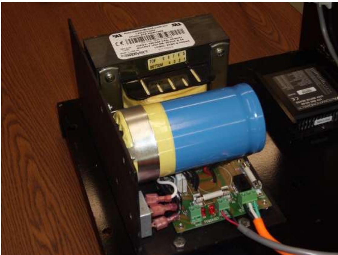
FIGURE 14. POWER SUPPLY USED TO CONVERT A.C. TO D.C.
