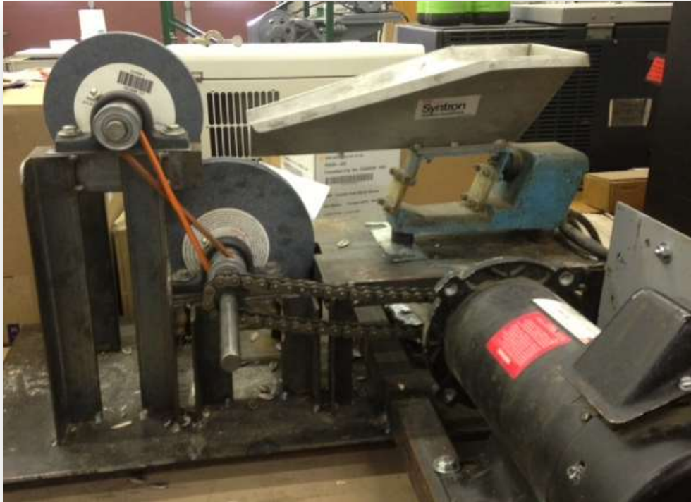
Figure 2. Counter-rotating grooved wheel prototype designed by Bob Majczak ready for evaluation.
