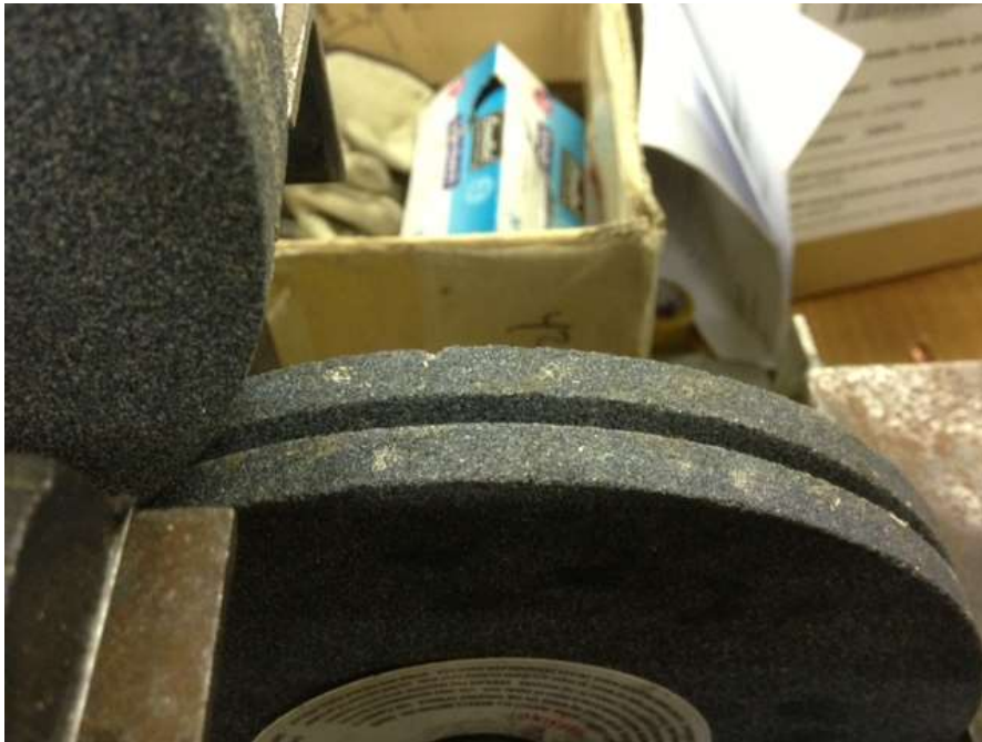
Figure 7. Bottom cracker wheel of counter-rotating wheel design with 1/8" groove.
