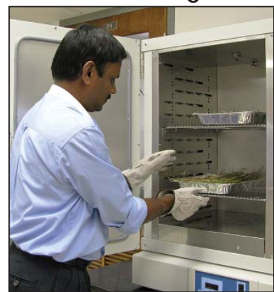
Dr. Igathi Cannayen carrying out mechanical drying studies on switchgrass biomass.
