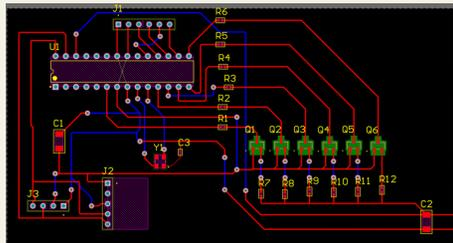
A 2-layer PCB made to prioritize a small profile when compared to previous prototypes. This version uses headers for most parts to allow comparison between different pieces of hardware without needing to manufacture a new board.
