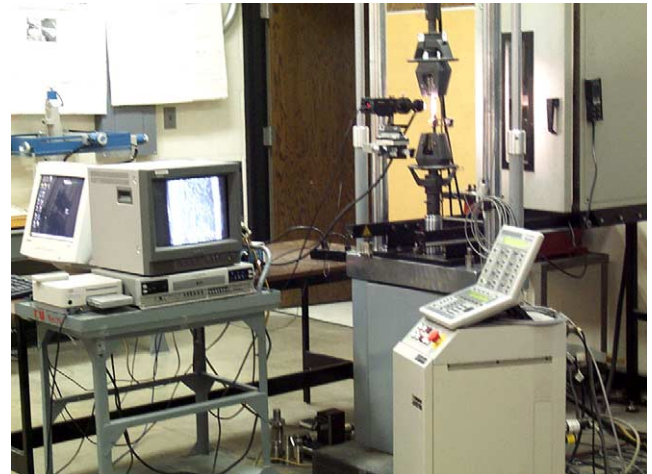
Fig. 8. Edge-delamination tensile testing setup.
