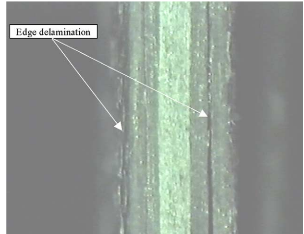
Fig. 11. Edge delamination along 12^\circ/-12^\circ interfaces.
