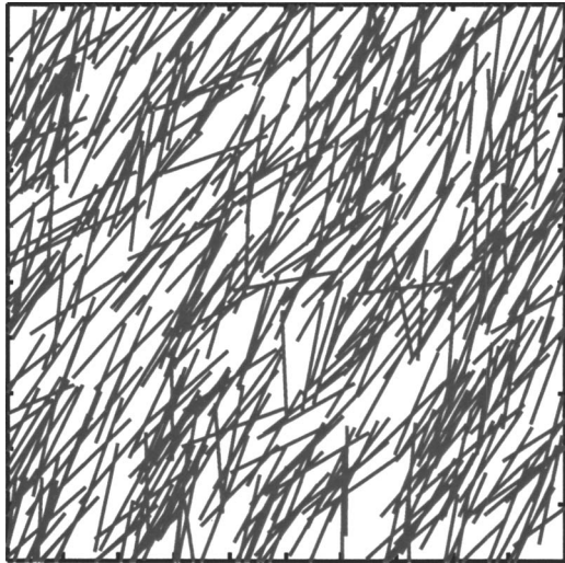
FIG. 2. Fiber network with preferred orientation. (Fiber concentration: 20 (in fiber length unit), mean orientation angle: 60^\circ , and standard deviation: 15^\circ ).
