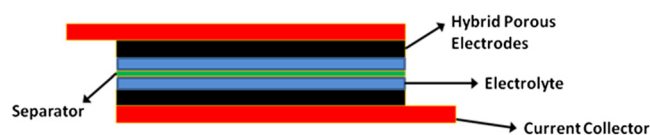
FIG. 2. (Color online) Schematic of a prototype supercapacitor made of hierarchical electrodes.
