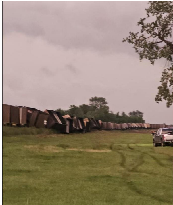
Figure 10: Derailed train caused by a tornado near Steele ND on August 28, 2024
