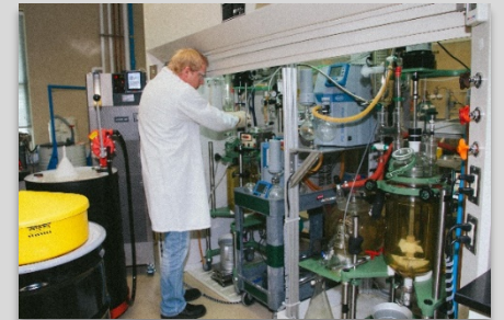
Scale-up reactor vessels to produce pilot project volumes.
