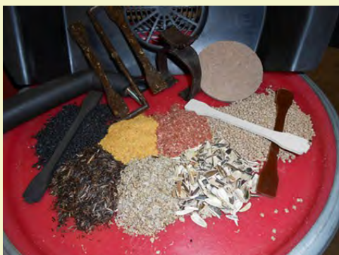
Examples of biocomposite materials used by c2renew that reinforce and strengthen plastics
