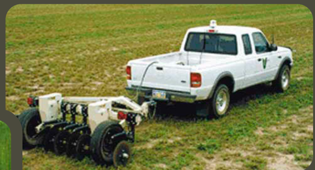
Veris soil EC sensor. (Photo courtesy of Veris Technologies, Salina, Kan.)
