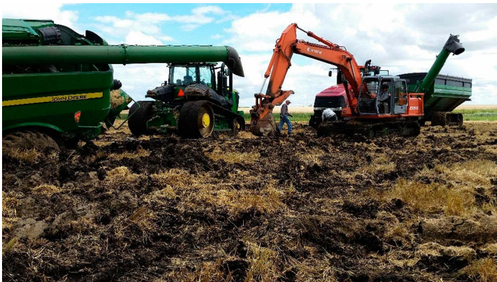
Figure 15. Digging out a buried combine harvester in the Devils Lake area of North Dakota during a wet fall. Soils were composed of significant illite, with smectite slightly dominant. The field is managed as conventional till. (NDSU photo)
