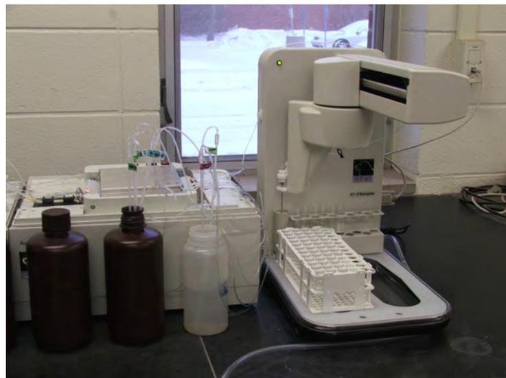
We have added an AA3 Segmented Flow Multi-Chemistry Analyzer, which will allow us to be more efficient and accurate in our soil testing practices.
