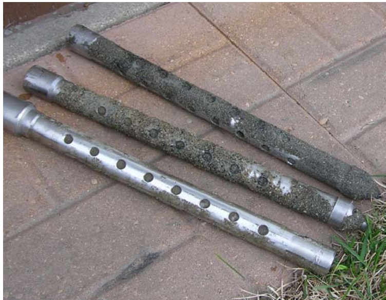
Figure 11. Photograph of one-foot stainless steel well screens pulled from the meadow (upper two screens) and dune (lower screen) monitoring site. Note the strong precipitation of calcite cement on the meadow points; points were in place for about 18 months.
