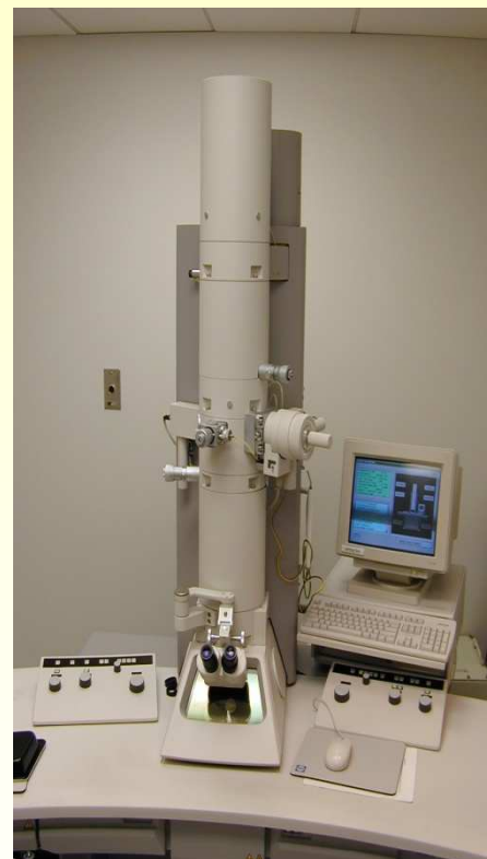
Transmission electron microscope (TEM) (size distribution of the nanoparticles)
