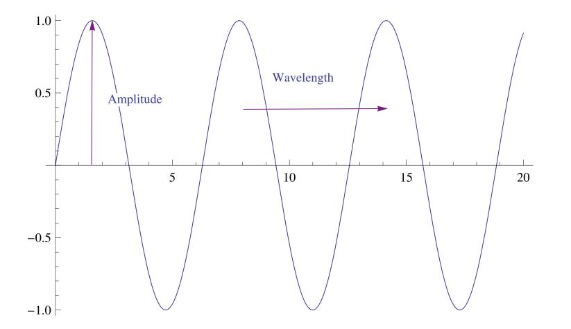
Meaning of wavelength and amplitude. The wavespeed is the speed at which a crest or a trough moves down the rope.
