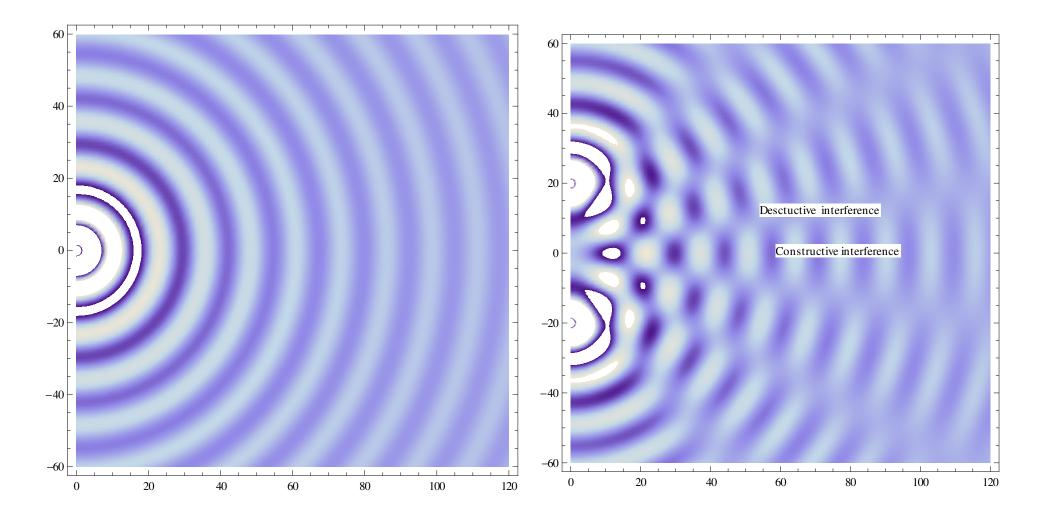
Overlapping of waves leads to interference. Most waves just add to each other: if valleys hit valleys and hills hit hills in time then the wave will be twice as big, but if valleys hit hills and hills hit valleys then the wave gets extinguished.
