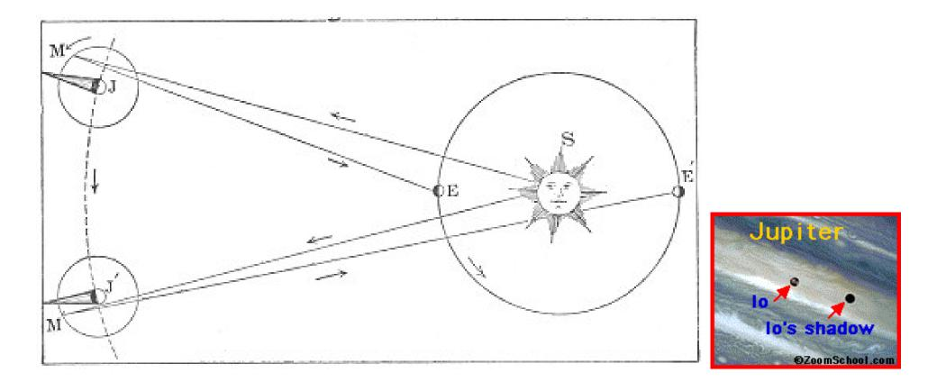
By looking at the apparent orbital speed of Jupiter's moon Io, we can see that there is a small but visible difference depending on Jupiter's and earth's relative position. This can be attributed to a finite speed of light if the speed of light is about  $3 \times 10^8 m/s$ .
