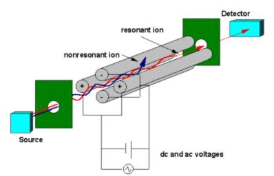
The quadrapole mass spectrometer as you can see has four parallel rods. To these rods is applied a alternating voltage with the function below:
