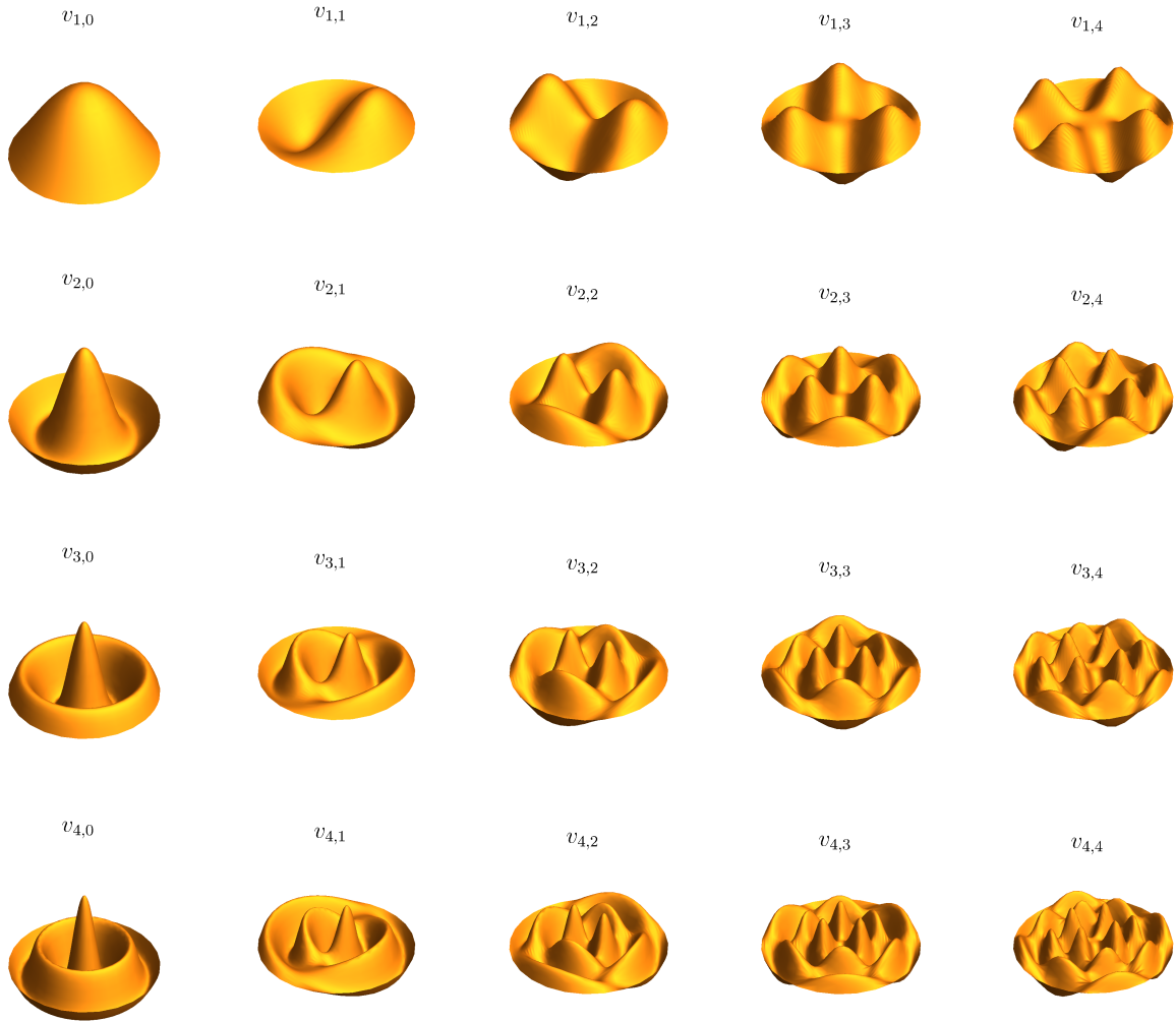
Figure 3: Fundamental vibrations (note that I am using the second index to denote the order of Bessel's function, and the first index to denote the k -th root, which is opposite to what is used in the textbook)
